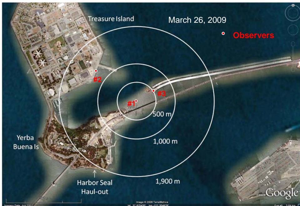
Figure 4: SAS temporary tower project area with 500 meter (preliminary), 1,000 meter (160 dB impact), and 1,900 meter (120 dB vibratory) MMSZs and marine mammal monitor observation sites for March 26, 2009.
