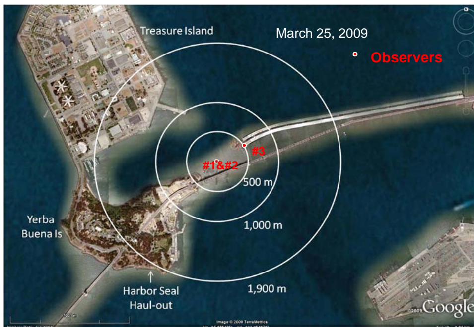
Figure 3: SAS temporary tower project area with 500 meter (preliminary), 1,000 meter (160 dB impact), and 1,900 meter (120 dB vibratory) MMSZs and marine mammal monitor observation sites for March 25, 2009.
