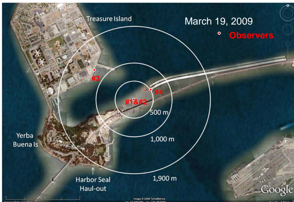
Figure 3: SAS temporary tower project area with 500 meter (preliminary), 1,000 meter (160 dB impact), and 1,900 meter (120 dB vibratory) MMSZs and marine mammal monitor observation sites for March 19, 2009.
