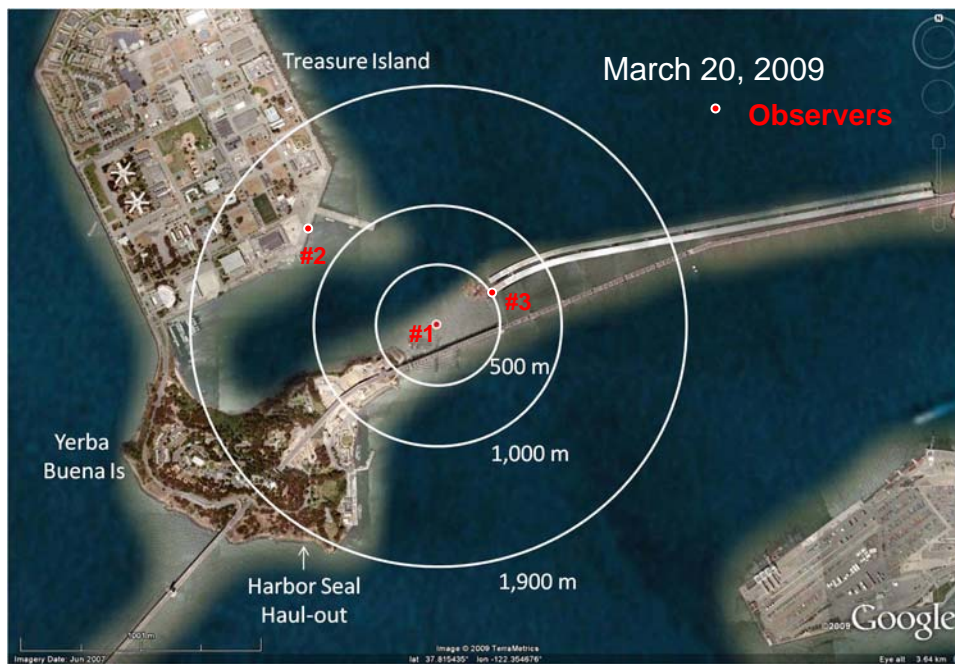
Figure 4: SAS temporary tower project area with 500 meter (preliminary), 1,000 meter (160 dB impact), and 1,900 meter (120 dB vibratory) MMSZs and marine mammal monitor observation sites for March 20, 2002.
