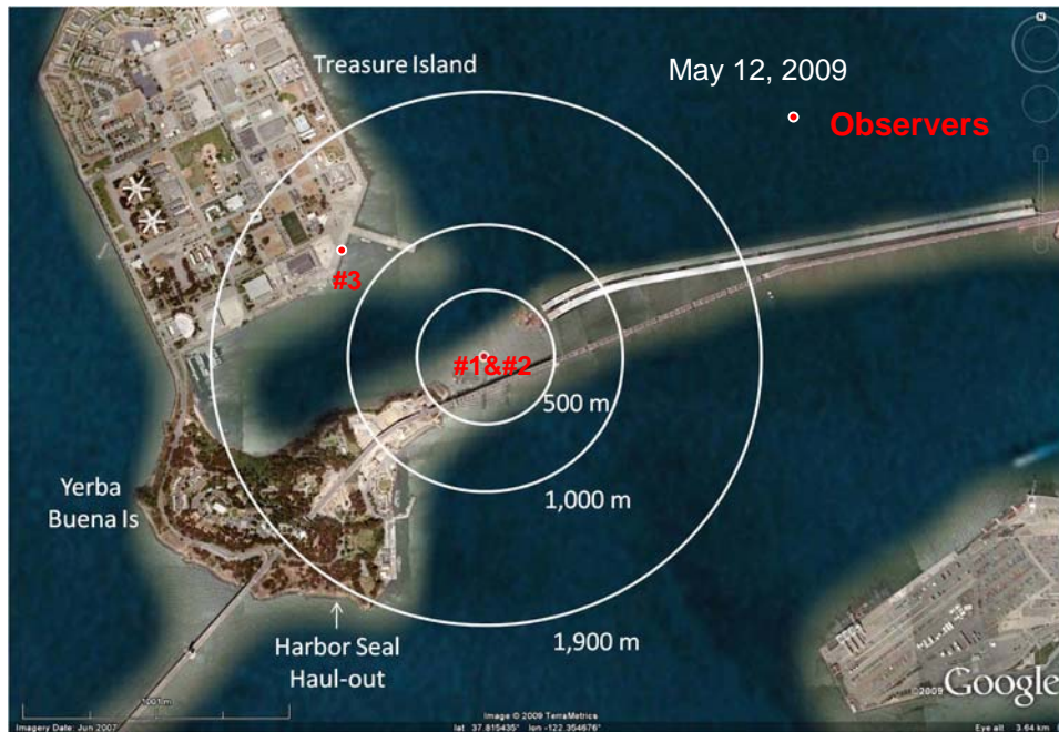
Figure 3: SAS temporary tower project area with 500 meter (preliminary), 1,000 meter (160 dB impact), and 1,900 meter (120 dB vibratory) MMSZs and marine mammal monitor observation sites for May 12, 2009.
