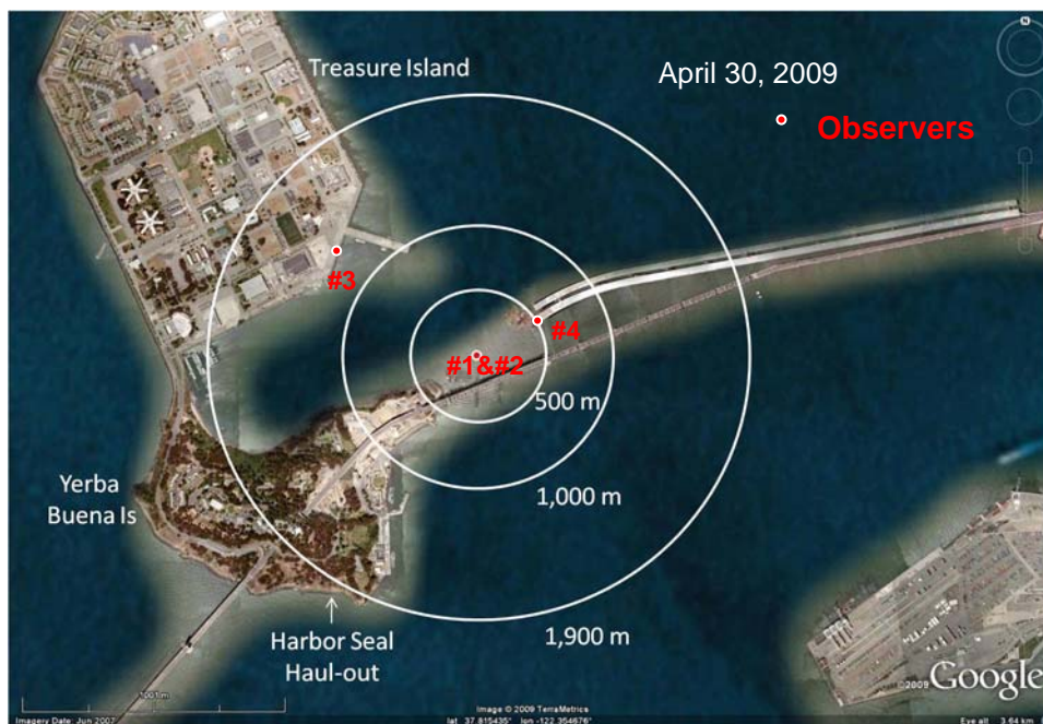
Figure 3: SAS temporary tower project area with 500 meter (preliminary), 1,000 meter (160 dB impact), and 1,900 meter (120 dB vibratory) MMSZs and marine mammal monitor observation sites for April 30, 2009.
